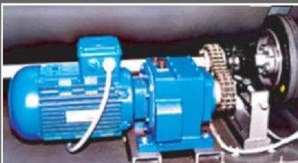
Totally enclosed motors are rugged and provide long life, meaning lint damaged motors are a thing of the past. The machine is provided with a soft start device for smooth starts and stops. Optionally, an inverter is available for more precise control.
